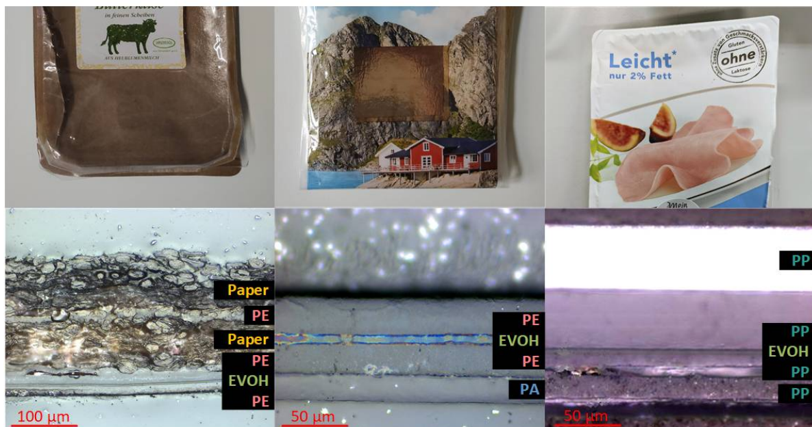
Figure 30: Packaging structure samples comprising a common barrier structure (PE-EVOH-PE) combined with paper (left), PA (middle) and PP (right).
