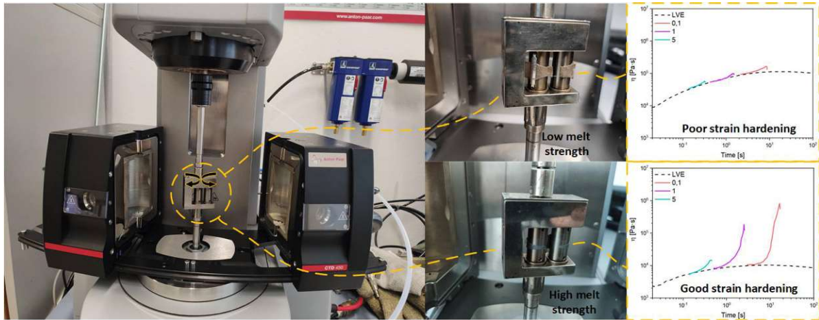
Figure 25: Extensional rheology measurement principle and polymer melt behavior
