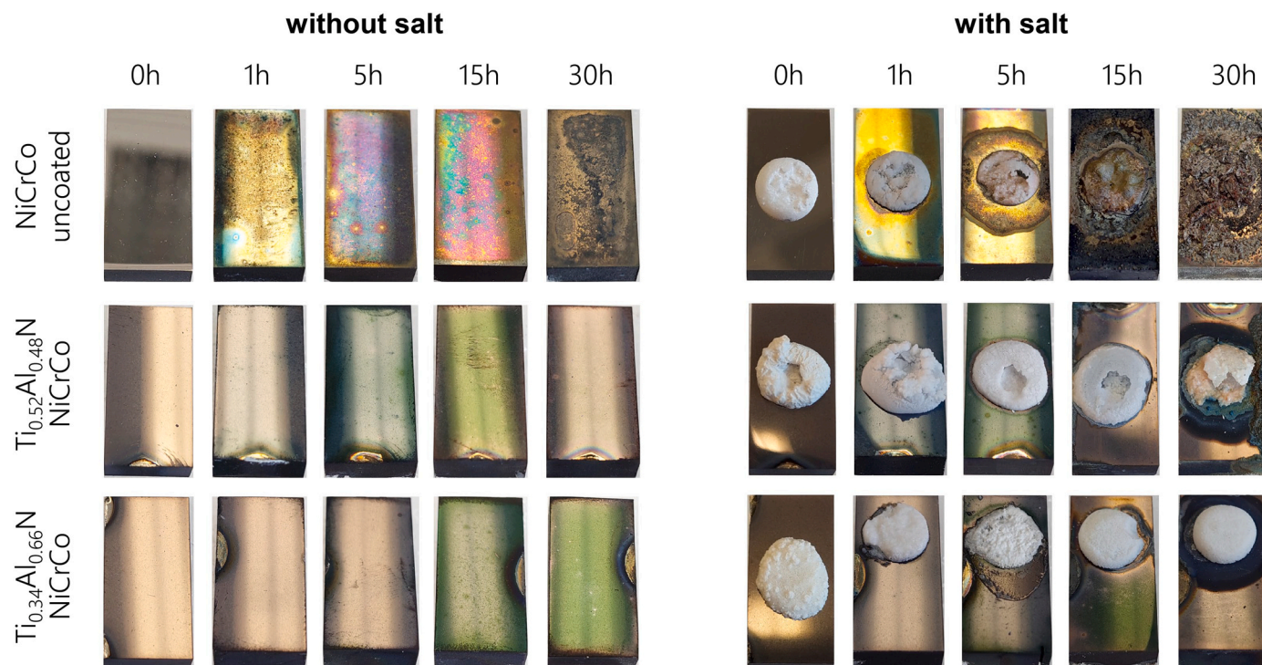
Fig. 3. Top-view images showing annealed samples at 700 °C in \text{SO}_x -rich atmosphere without salt-deposits for 0, 1 h, 5 h, 15 h and 30 h (left group), as well as annealed samples with salt-deposits under identical conditions (right group). The first row features uncoated Nimonic c-263 substrates, while the second and third row show \text{Ti}_{0.52}\text{Al}_{0.48}\text{N} and \text{Ti}_{0.34}\text{Al}_{0.66}\text{N} coated c-263 substrates, respectively.
