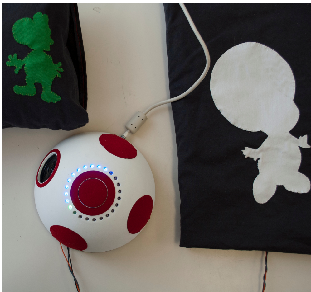
Figure 4.18: The Rattle Alarm System – Developed together with Mia – left: cushion, middle: alarm clock, right: pressure mat
