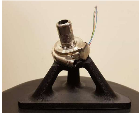
Figure 15: A prototype for the pump holder, which defines the direction and position of the LVAD within the MCL.
