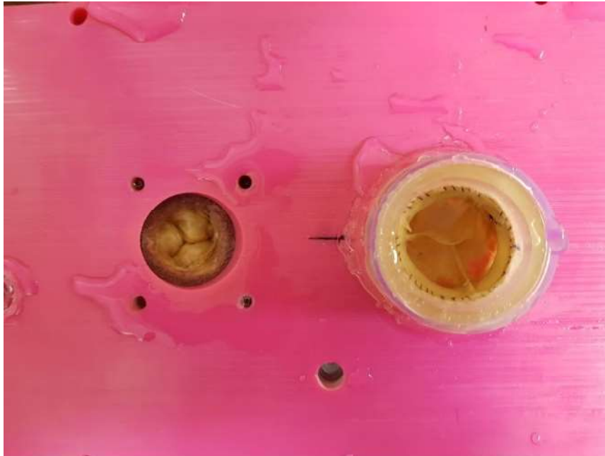
Figure 20: The biological valves were placed inside cylinders in the MCL lid. The orientation of the leaflets was chosen carefully and aligned with an indication on the lid. The mounting of an additional LVOT is possible on the left, where the AV is placed in a recess of the lid.
