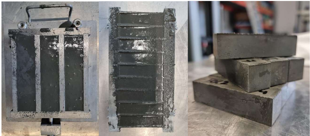
Figure 4.4: Standard sample molds (left), Small sample molds (middle), samples removed from molds after 24 hours (right)
