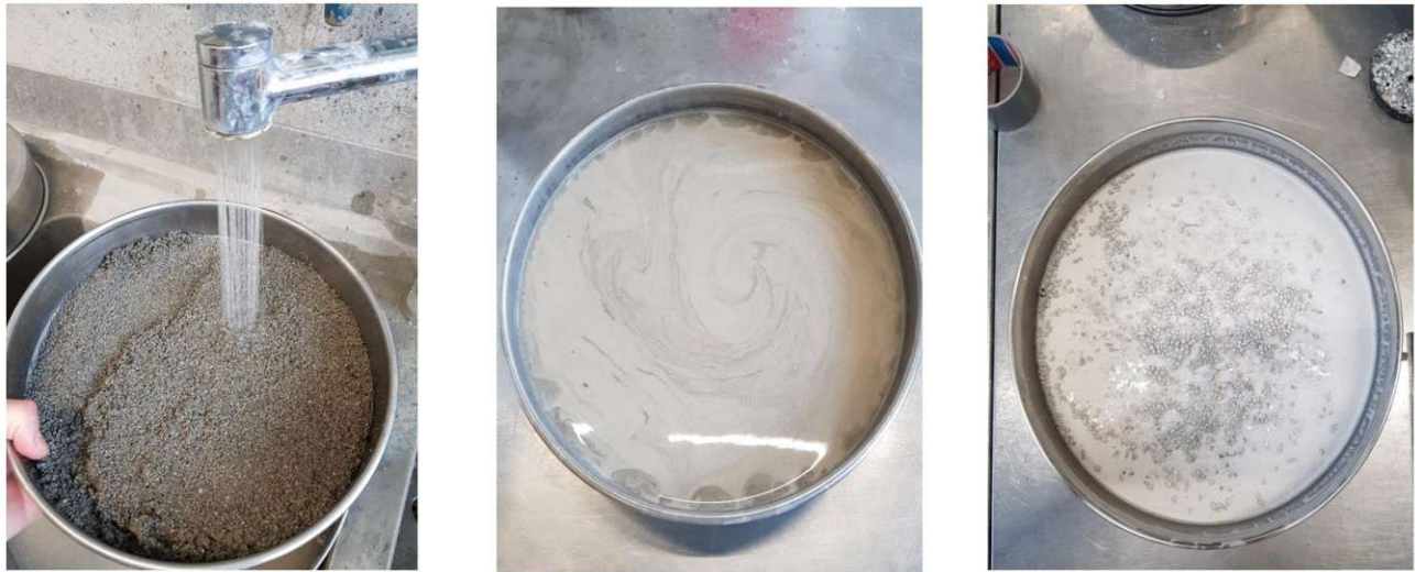
Figure 3.5: Evaluation phases of the dust content: Washing the aggregate (left); collected water and dust before drying (middle); residual dust after drying (right)
