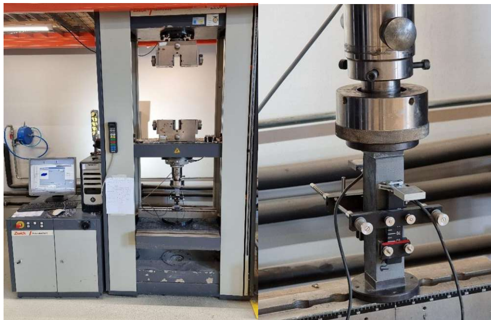
Figure 4.8: Apparatus for assessing the E-Module (left); Sample during testing (right)
