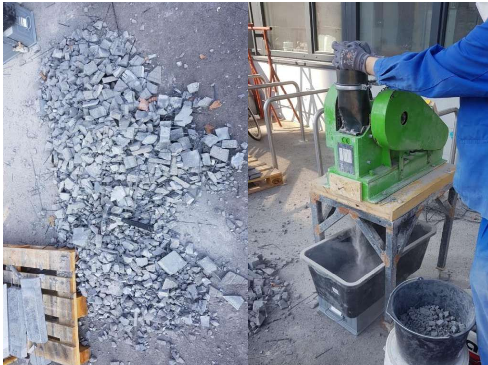
Figure 1.1: Breaking of UHPC samples (left); grinding with the help of the machine (right)
