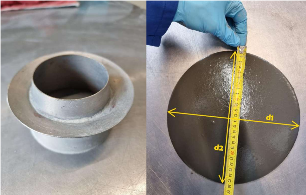
Figure 4.1: Metal slump cone (left), concrete spread (right)
