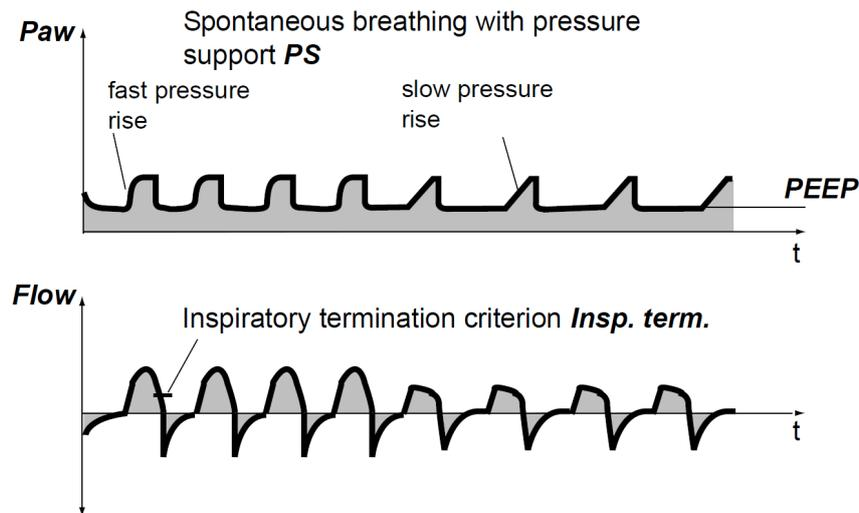
**Fig. 3.4.1.:** If the patients breathing effort is sufficient, a preset pressure support will be applied by the ventilator in order to facilitate the breathing effort of the patient. Image taken from [47].
