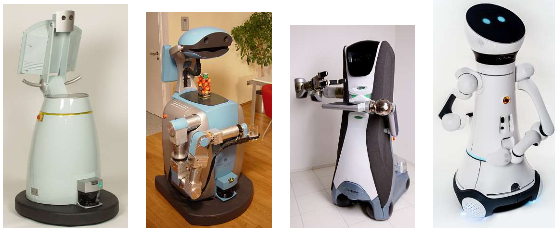
Figure 2.3: Care-O-Bot designs from first to fourth generation (left to right). Image sources: https://www.care-o-bot.de/en/care-o-bot-3/history/care-o-bot-i.html https://www.care-o-bot.de/en/care-o-bot-3/history/care-o-bot-ii.html https://www.care-o-bot.de/de/care-o-bot-3/download/images.html , https://www.care-o-bot.de/de/care-o-bot-4/download/images.html
