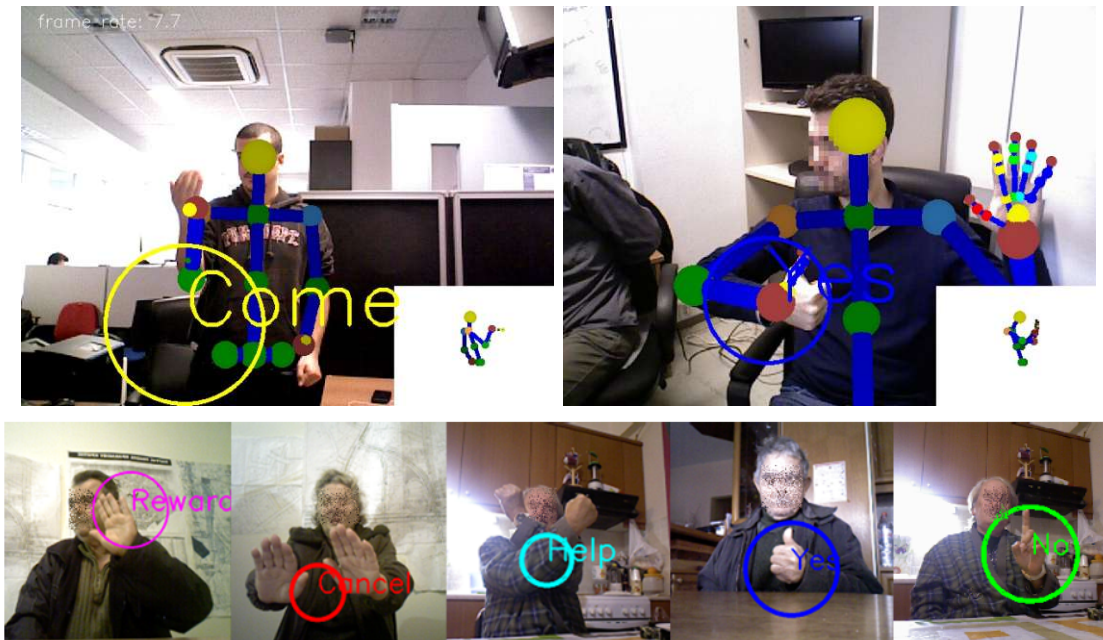
Figure 4.10: Integrated human body detection and tracking and gesture recognition. The output of the former module feeds the gesture recognition method based on 3D position and angles of the tracked body joints. Left: “Come closer” gesture of a standing person. Right image: “Yes” gesture of a sitting user. Lower image was previously reported in [Michel et al. [77]]
