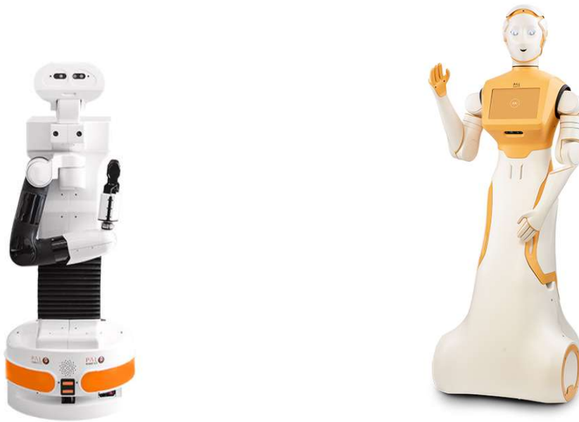
Figure 2.5: PAL Robotics TIAGo (left) and ARI (right). TIAGo is designed for a variety of applications, such as logistics, retail, and education, ARI is useful in education, healthcare, and customer service applications. (Image sources: https://pal-robotics.com/robots/tiago/ , https://twitter.com/PALRobotics/status/1463449099773095944 )
