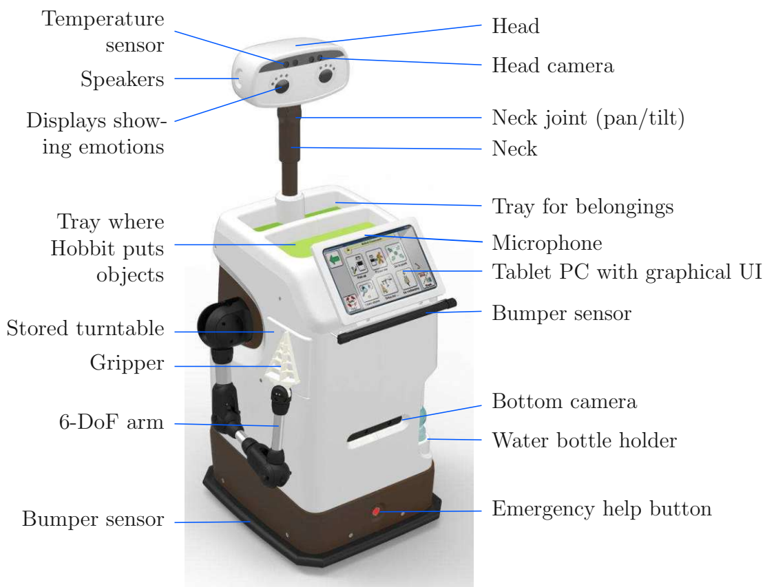
Figure 4.2: Rendering and hardware description of the second prototype of Hobbit (PT2).
