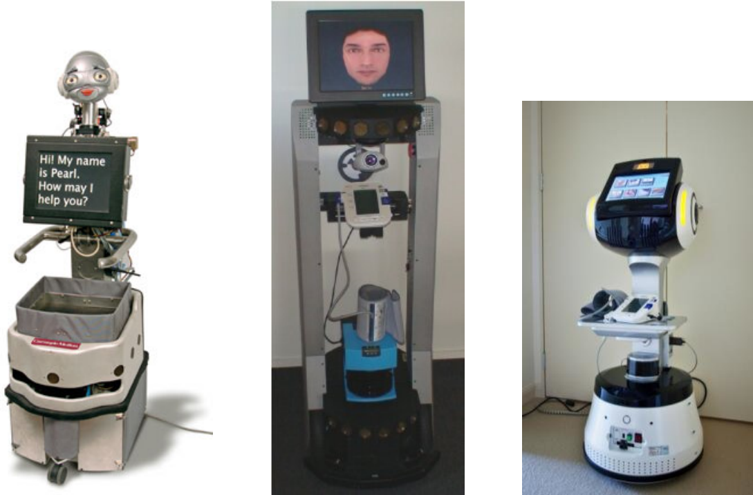
Figure 2.2: Pearl's ability to project a persona relies on essential elements such as the configurable head, including the size and spacing of her eyes, as well as the shape of its lips. The integrated basket of the robot enables easy transportation of objects by placing them inside it. (Image source: https://www.cmu.edu/cmtoday/issues/dec-2004-issue/feature-stories/human-health/index.html ) (left); Charles is outfitted with a diverse array of hardware components, including a differential drive system, SICK laser range finder, and sonar and infrared sensors. (middle); The Healthbot robot incorporates a touch screen, camera, speakers, and microphones to facilitate input and output interactions. It utilizes a Hokuyo LIDAR for navigation, allowing it to effectively perceive its environment. Additionally, the robot includes a blood pressure meter, offering the capability to monitor this vital sign as part of its functionality. (Image source: [Stafford [104]]) (right)
