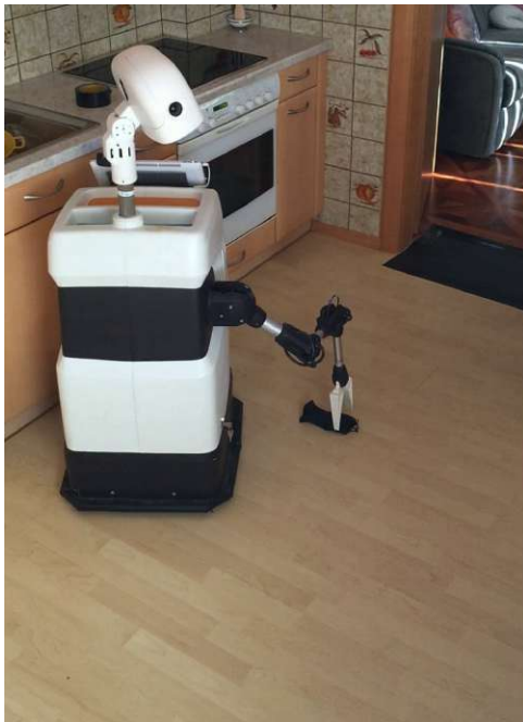
(c) After the object was detected, and grasping points were calculated, Hobbit grasps the object.
