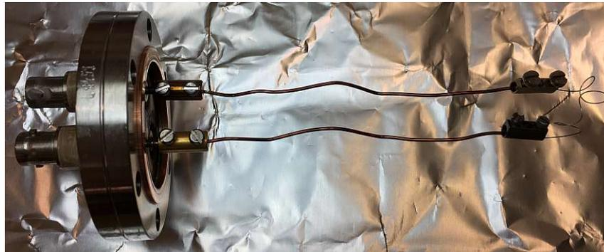
**Figure 17:** Photo of the tungsten wire feedthrough construct for the ultimately used test rig setup. It was constructed in such a way that the tungsten wire ended up right in front of the EA10+ opening.
