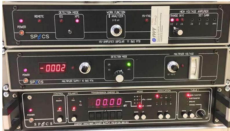
**Figure 9:** The front panels of the three rack-mounted electronic units of the EA10+. From top to bottom, the high voltage amplifier, the multiplier power supply, and the energy analyzer power supply are shown. The defined parameters are the ones which are automatically set by default when the units are turned on.
