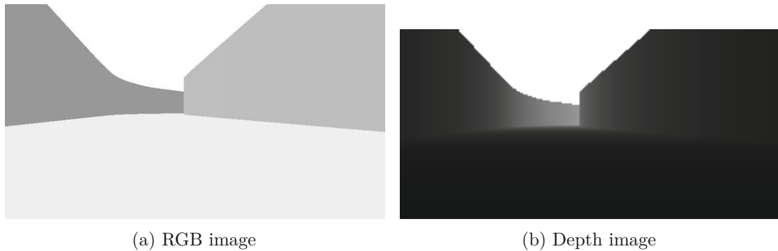
Figure 5.2: Visual inputs provided by the simulation environment. Both pictures show the same scene but with slightly different fields of view, and the depth image in each pixel shows the distance from the sensor to the first solid object. In the depth image, lighter values indicate higher distances.
