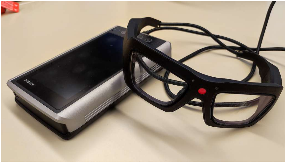
Figure 3.1: VPS19 Smart Unit (left) and eye-tracking glasses (right) used for eye-tracking in this thesis. This eye-tracking device records the wearer’s gaze and a video stream from the center of the field of view (light circle in the middle of the glasses).
