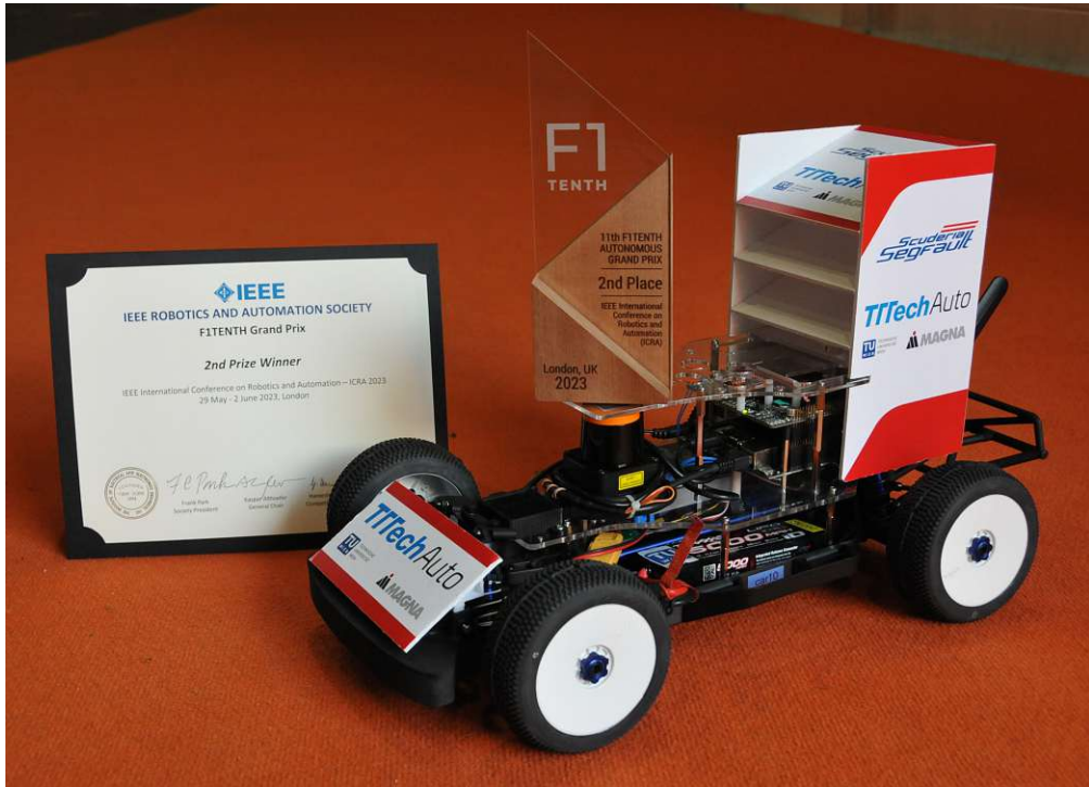
Figure 3.2: F1Tenth racing car from Vienna Technical Universities team used at the 11th F1Tenth Grand Prix at ICRA 2023 in London. The car performs all calculations with the onboard computation unit and uses LIDAR and inertial sensors for navigation.
