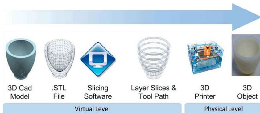
Figure 3: AMT process flow 6
