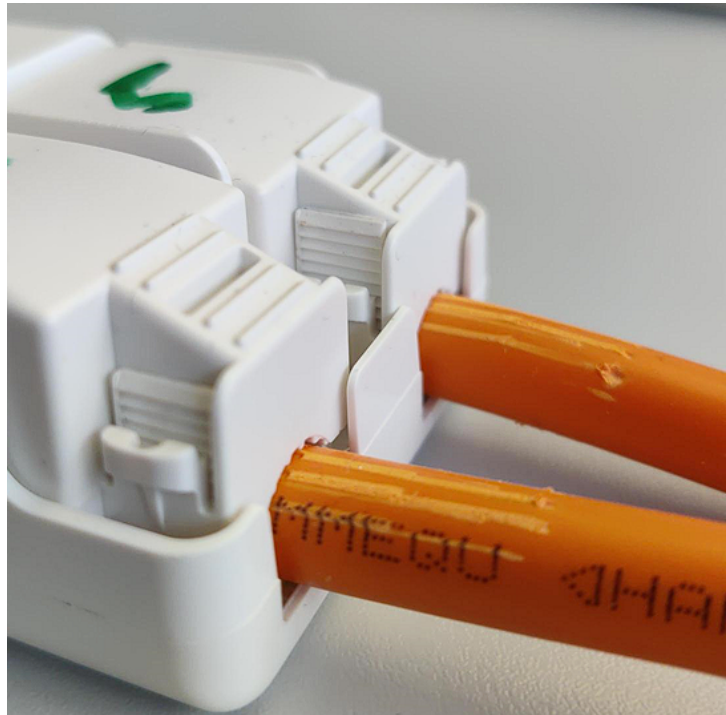
Fig. 2.12: System after a pull-out test
