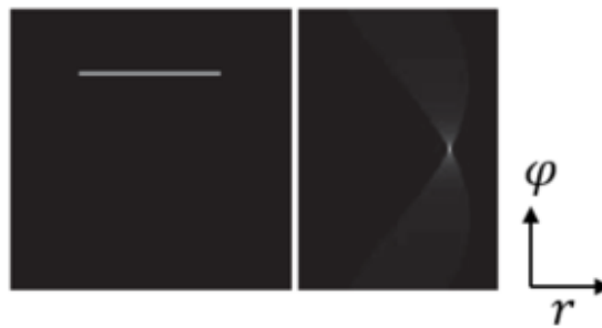
Figure 8. Simple example of the sinogram of a line [24]. The abscissa of the sinogram is the orthogonal distance r to the center and the ordinate is the projection angle \varphi [24].
