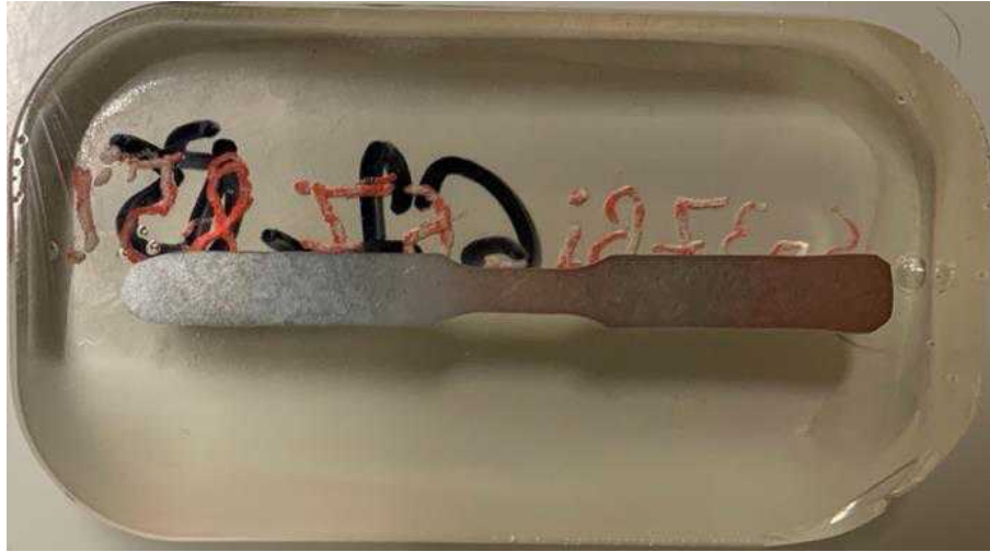
Figure 46: Damaged solder sample embedded in slow curing resin after grinding and polishing
