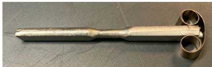
Figure 49: Dog bone shaped solder sample
