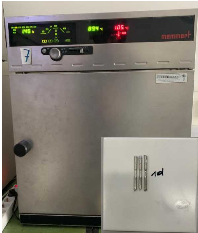
Figure 56: Oven used for long-term stability test on air; Insert shows tile with samples.
