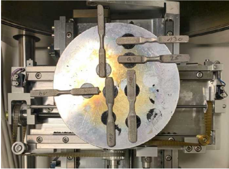
Figure 51: Attachment of 6 samples on a conductive plate in the SEM microscope
