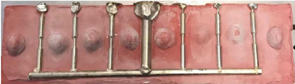
Figure 39: 6 solid solder samples after molding process in a high-temperature silicone mold
