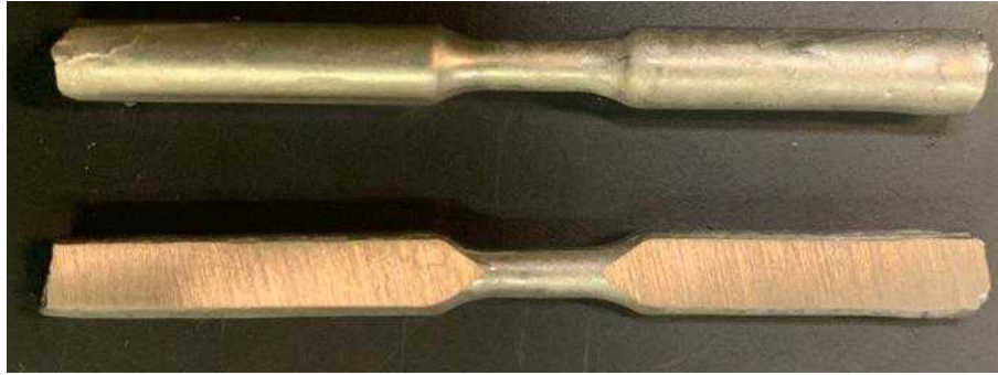
Figure 41: A solder sample before (upper) and after (lower) machining in its final form.
