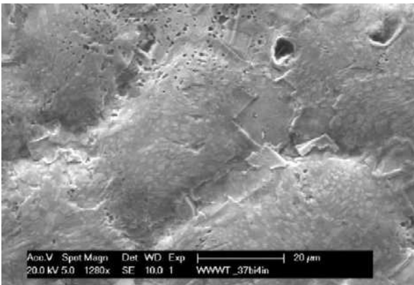
Figure 104: SE image of the top side of a „130 °C“-sample with 1280 times magnification with typical rectangular Bi crystals in between the homogenous matrix
