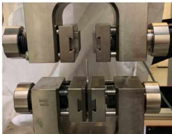
Figure 57: Clamped sample in Zwick/Roeller Z250 tensile/compression machine
