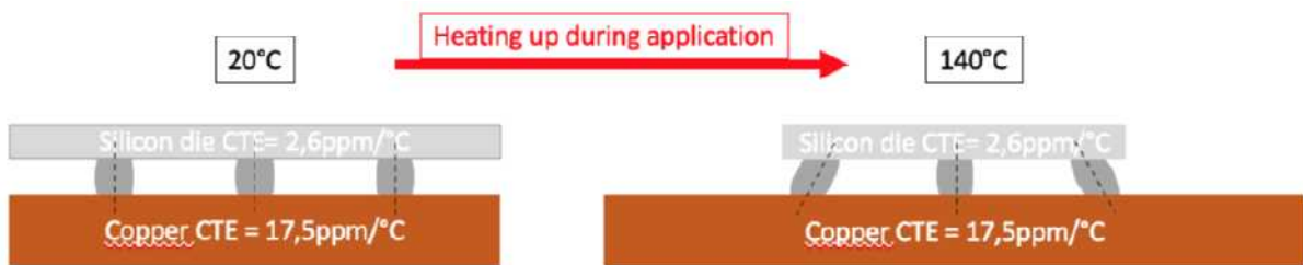
Figure 6: Illustration of CTE mismatch during application
