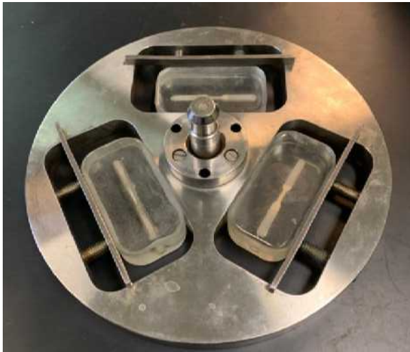
Figure 47: sample holder with three chucked samples
