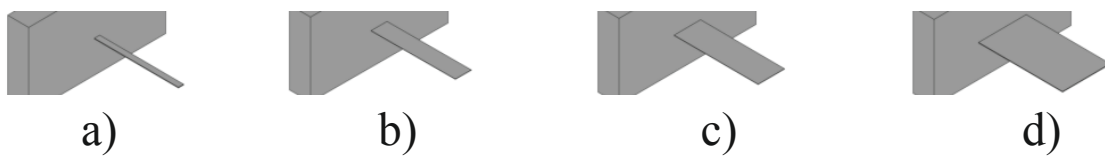
Figure 11.1: Example of plates with different widths a) b = 15 \mu\text{m} , b) b = 100 \mu\text{m} , c) b = 200 \mu\text{m} and d) b = 400 \mu\text{m} here investigated.
