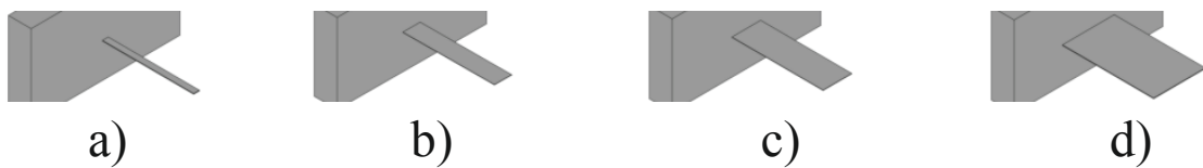
Figure 6.1: Example of plates with different aspect ratios a) r_a = 64/1 , b) r_a = 64/12 , c) r_a = 64/20 and d) r_a = 64/32 which are here investigated.
