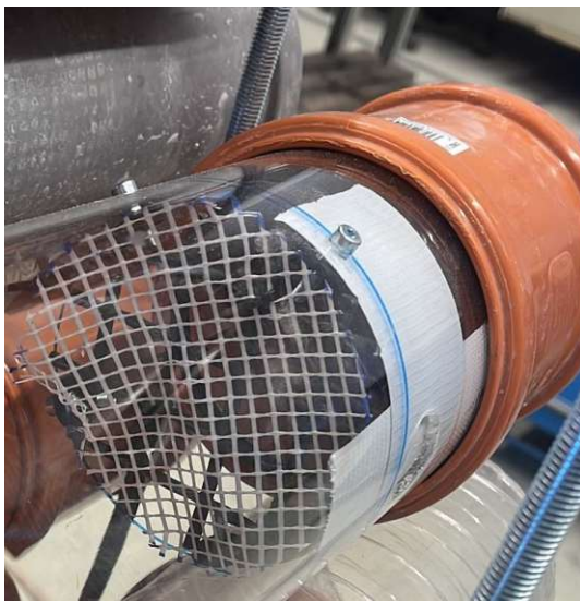
(a) Mesh to fix the beads in the pipe
