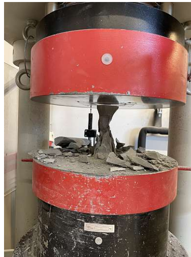
Fig. 2.24: Compressive strength test.
