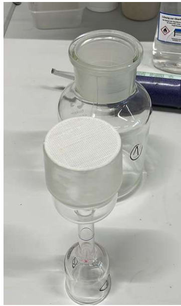
Fig. 2.17: Pycnometer with mesh.
