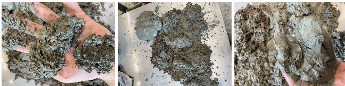
Fig. 4.7: Consistence slurry. Fig. 4.8: Different consistence in the pipe. Fig. 4.9: Material downwards the mesh.
