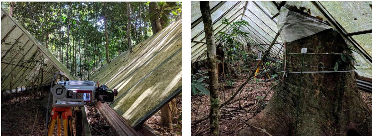
Figure 1 Illustration of the drought experiment and the RIEGL VZ-400 terrestrial laser scanner.
