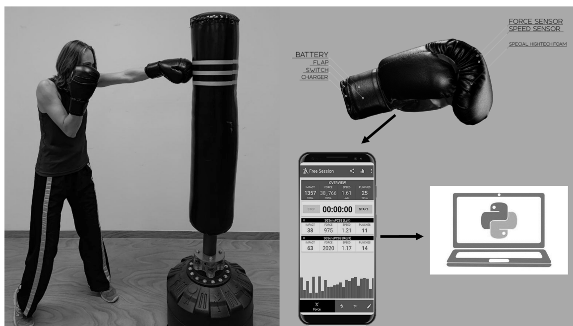
Figure 3. System setup with the punching bag target. The RD \alpha gloves send the sensor data via Bluetooth to the mobile app. The data are subsequently processed via Python for model implementation.
