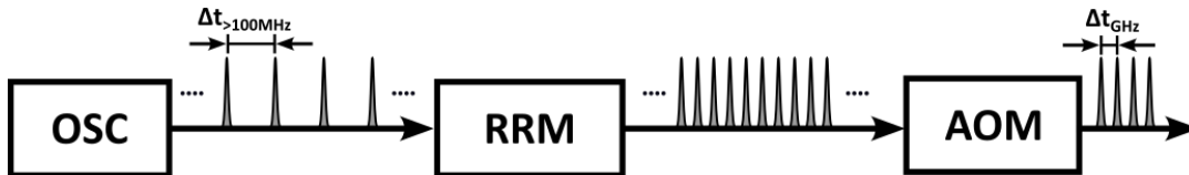
Figure 2.1: A typical method to generate ultrashort pulse bursts with GHz intraburst rates.
