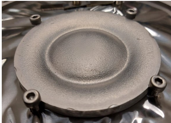
Figure 3.3. Racetrack on a target after magnetron sputtering.
