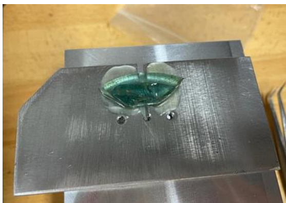
Figure 3.2: Sample fixed on metal plate before cutting
