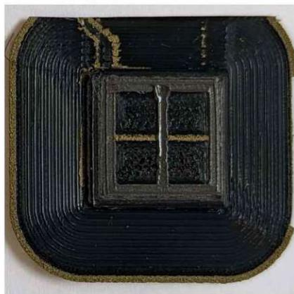
Figure 66: Printed sample cross structure made of filaments doped with steel (bottom) and brass (top) on a pure polymer support structure. The quadratic printed structure is approximately 1 *cm* wide with a layer thickness of 60  $\mu\text{m}$ .
