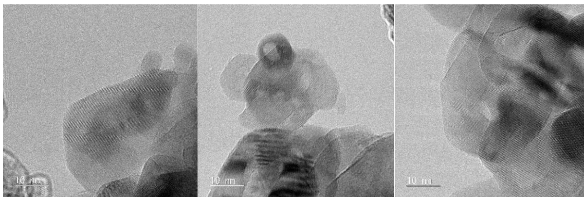
Figure S6: TEM pictures corresponding to \text{Cu}(\text{ac})_2/\text{TiO}_2 ranging from non-calcined to 400 °C (left to right).
