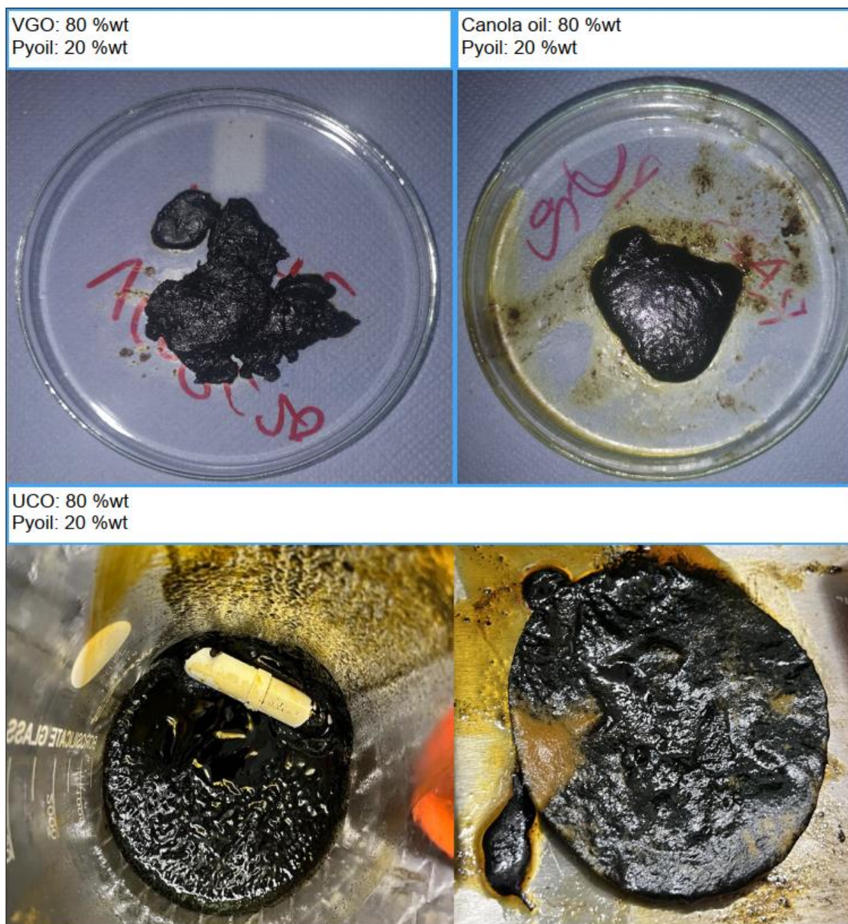
Figure 21: Precipitation of the VGO/UCO/canola oil and pyoil admixtures
