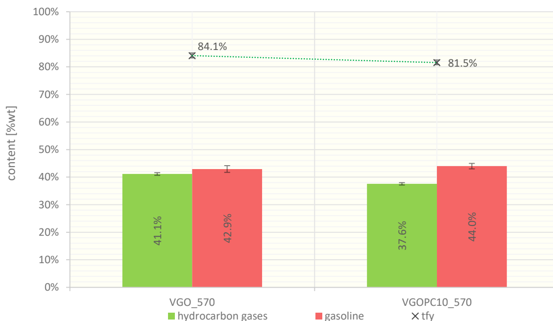
Figure 53: Hydrocarbon gases, gasoline yield and tfy of high severity cracking experiments with VGO and 10 %wt pyoil
