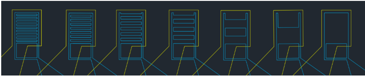
Figure 31 Cantilever structures with ladder-like electrode design to achieve higher field gradients. Designs with decreasing ladder steps are shown from left to right. Importantly, each ladder design has the same electrode area. This figure does not show the actual positions of each cantilever design but was ordered side by side for illustration purposes.
