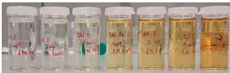
Figure 6-17 Ammonia detection via Nessler's reagent method: a) UV-Vis absorption curves of different concentrations of  $NH_4^+$  ions using Nessler's reagent method; b) A calibration curve used to estimate the concentrations of  $NH_4^+$  ions; c) Standard solutions of different  $NH_4^+$  concentrations.
