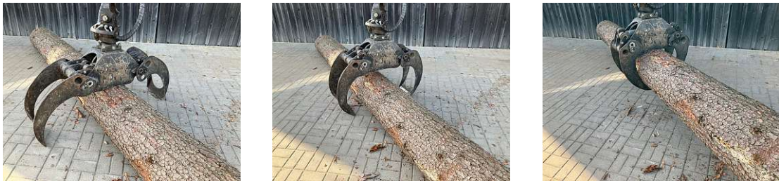
Figure 4.2: Grasping a log from the ground.
