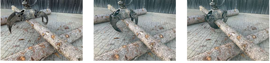
Figure 4.3: Grasping a log on supports.
