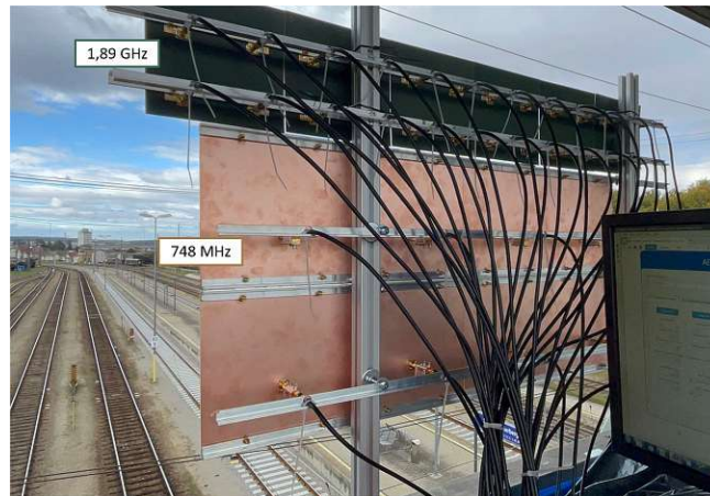
Figure 4.1: The AIT massive-MIMO channel sounder from the footbridge.
