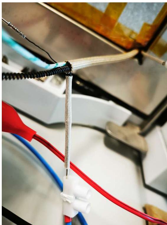
Figure 13: Close up of the transferline for the cooling tower setup.
