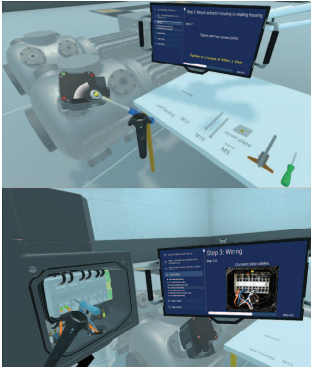
Figure 1: VR training setting. All assembly parts and tools are lying on the table. The required actions are described on the blue monitor. On the screenshot a screw is being tightened with a wrench (top). Users had to connect wires according to a picture in an enlarged copy of the housing (bottom).
