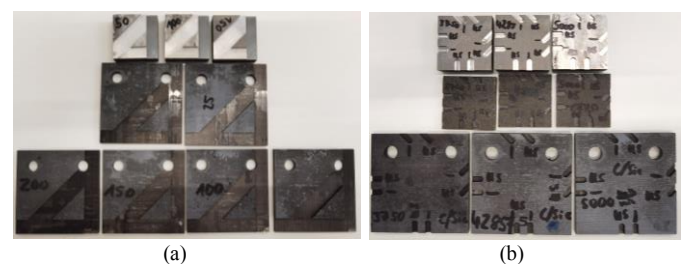
Fig. 3. (a) Top surface - flat ground composites; (b) Bottom surface - deep ground composites.
