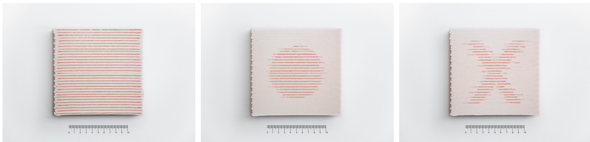
Figure 5. Sanded test specimens comparing consistent printing settings ( left ) with the successful positioning of the inside material according to multiple user-defined patterns such as circular arrangement ( center ) and crossed arrangement ( right ).
