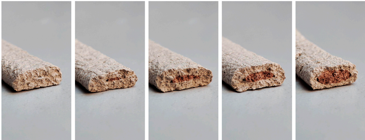
Figure 6. Cross-sections of different material compositions within one extrusion. From left to right, Mixtures 1, 2, 3, 4 and 5 as described in Table 2.
