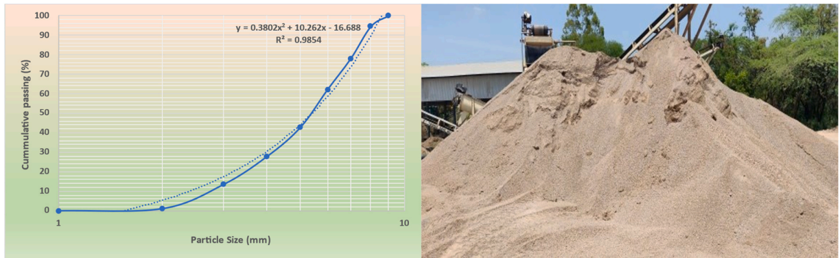
Fig. 5. Particle Size Curve and Washed Sand at Construction and demolition waste plant.
