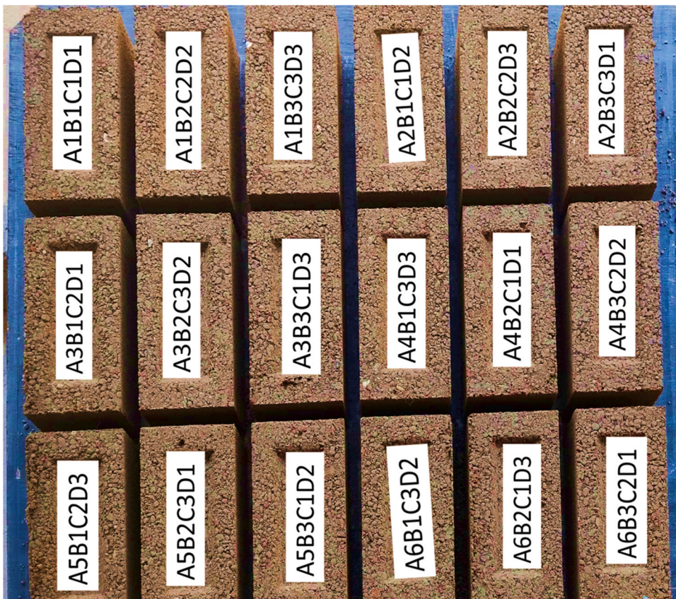
Fig. 11. Geopolymer Brick produced as per DOE.
