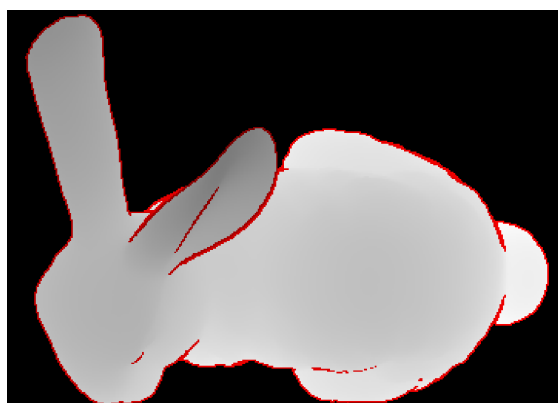
Figure 3.5: Range scan image with occlusion pixels marked in red.
