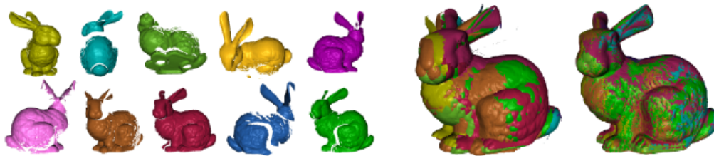
Figure 1.1: Several range scans, here shown as triangular meshes, being registered onto each other. First aligned roughly in a crude registration step, followed by fine registration. Image courtesy of Gelfand et al. [15].
