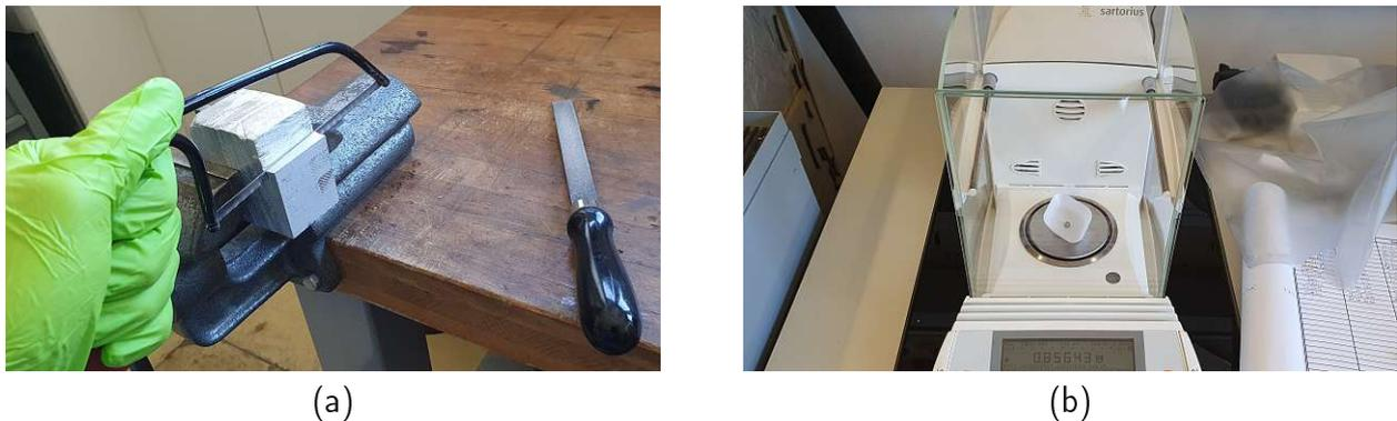
Figure 3.1: (a): Cutting pieces out of the aluminium block using a special saw blade. (b): Precision weighing vanadium using a Sartorius scale.
