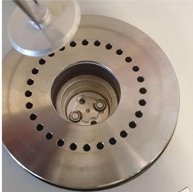
Figure 3.14: Sample holder for specific heat( $c_p$ )-measurement.
