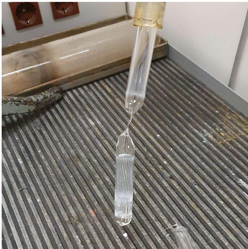
Figure 3.3: Quartz glass containing sample getting evacuated and then sealed via melting.
