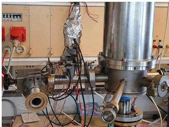
Figure 3.12: Outer shield with valves for the vacuum pump and helium pipe.
