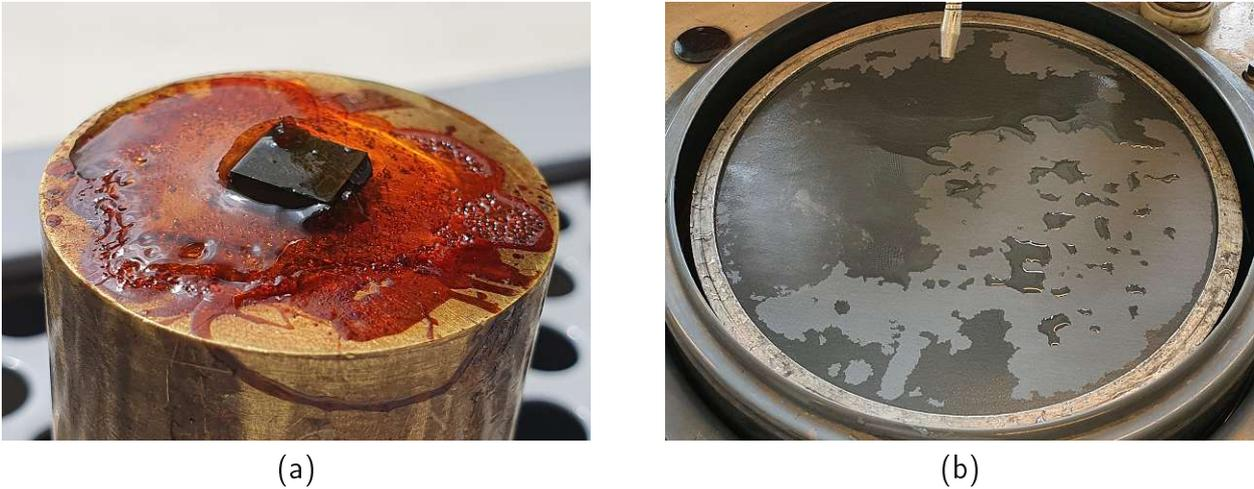
Figure 3.17: (a): Sample embedded in wax prepared for sanding. (b): Struers Planopol-2 polisher
