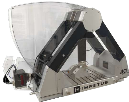
Figure 5: The impetus pendulum by 4a engineering GmbH is used for multiple material tests, which form the basis for the material card development. (retrieved from https://www.4a-engineering.at/4a-impetus )
