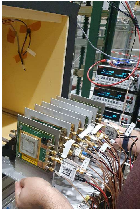
Fig. 10.2. Open cold box with with 5 DUTs and 2 LGADs mounted.
