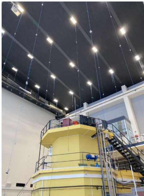
Figure 7: 3D monitoring matrix for airborne HTO investigation in the reactor hall of TU Wien
