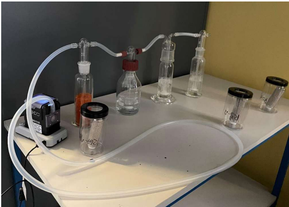
Figure 3: Active and passive monitoring instruments used in the co-comparison experiment [45]
