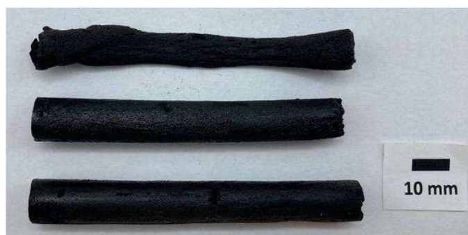
Figure S2: Silicon oxycarbide monoliths 7b prepared for continuous-flow experiments before cutting 15 mm pieces. Solid loadings of a) 10 b) 20 and c) 30 wt.% polysiloxane 1 in tert -butyl alcohol 3 were investigated, whereas b) 20 wt.% were used for all continuous-flow experiments.
