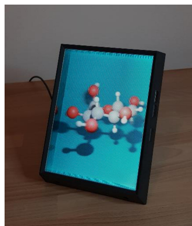
Figure 2. Visualization of a glucose molecule on a compact multi-view autostereoscopic display. The image reveals artifacts stemming from the employed parallax barriers, but these artifacts are notably less pronounced when viewed directly with the naked eye.
