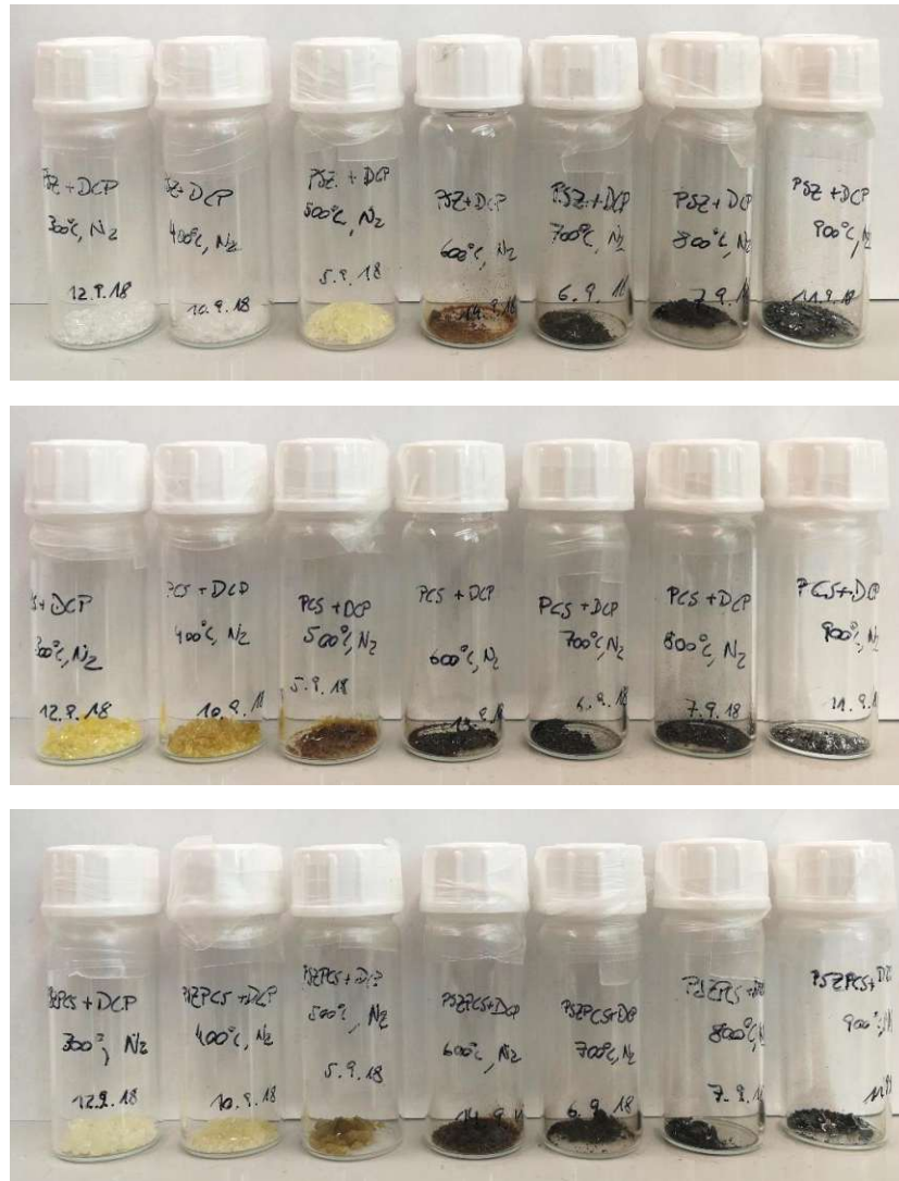
Figure 113: Sample images of PSZ (top), PCS (middle) and PSZPCS (bottom) after pyrolysis from 300-900 °C under nitrogen.
