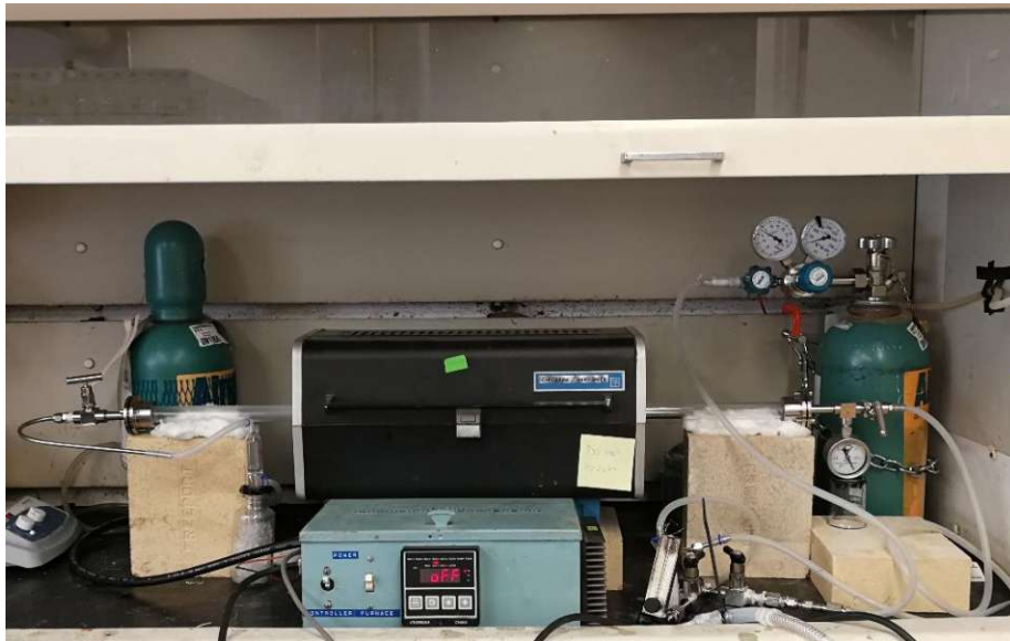
Figure 112: Furnace set up for the experiments using diluted ammonia.
