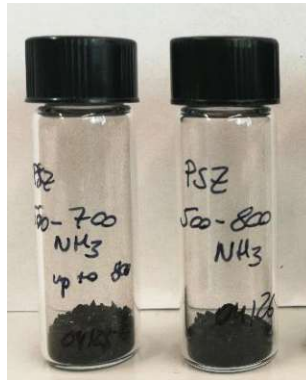
Figure 128: Sample images for PSZ treated with ammonia during a temperature window of 500-700 °C (left) and 500-800 °C (right) and up to a maximum temperature of 800 °C.
