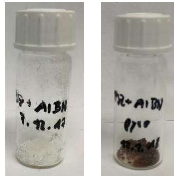
Figure 80: Sample images of the sample after crosslinking at 130°C with AIBN as initiator (left) and after pyrolysis at 600°C (right)
