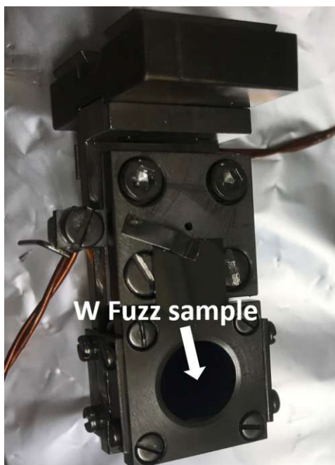
Figure 5.10 – W Fuzz sample inside the target holder.
