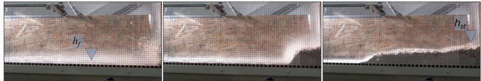
weight per unit area of  $2.8 \text{ kg/m}^2$ , and a tensile strength of  $2.94 \text{ kN/m}$  transverse to the direction of the embankment and  $1.37 \text{ kN/m}$  along the direction of the embankment. Figure 7 (right) shows the reinforced embankment in the slide.
