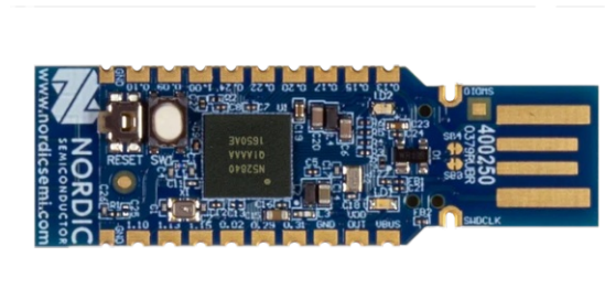
Figure 4.4: NRF52840 Dongle, [Norb]
