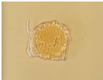
Figure 60: Printed part immediately after the exposure test with signs of overpolymerization
