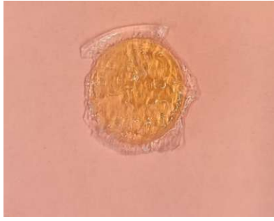
Figure 62: Printed part immediately after the exposure test with overpolymerization.
