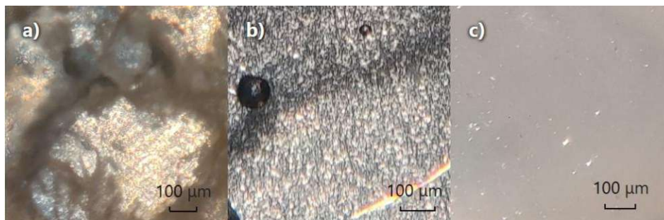
Figure 54: Phases of the 50APF polymer observed on the polarized optical microscope: a) room temperature, b) 115 °C, c) 133 °C.
