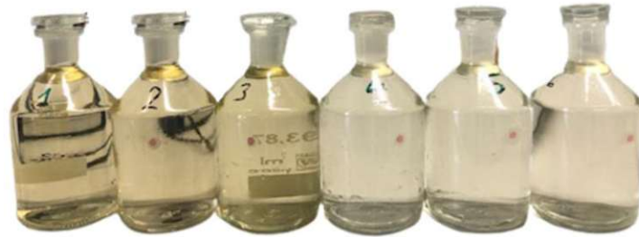
Figure 6: Used BOD flasks; the bleaching effect by O 3 is visible: three left BOD flasks contain sample, three right BOD flasks contain ozonated sample with a specific O 3 dose of 0.40 g O 3 g -1 DOC
