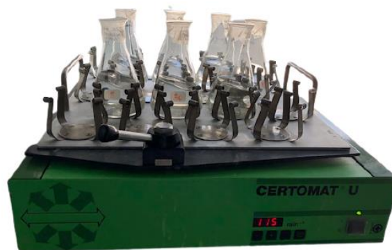
Figure 9: Adsorption experiments using the orbital benchtop shaker CERTOMAT® U; t_{eq} = 18 h; T = 23^\circ C
