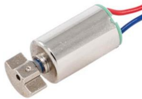
Figure 10: Small vibrator, to prevent cells from settling
