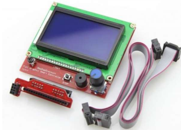
Figure 26: Kingprint LCD 12864, graphic smart display controller
