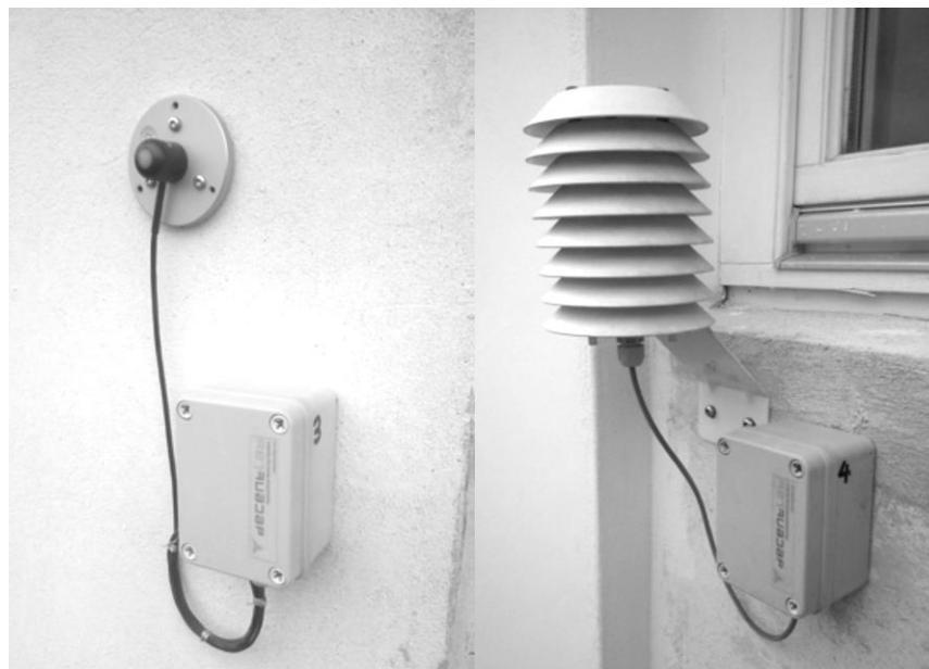
Figure 16: The solar radiation and temperature / humidity sensors (Schuss et al. 2017)
