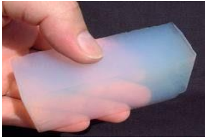
Figure 2: Examples of translucent Silica aerogel insulation block form (Berardi 2015)
