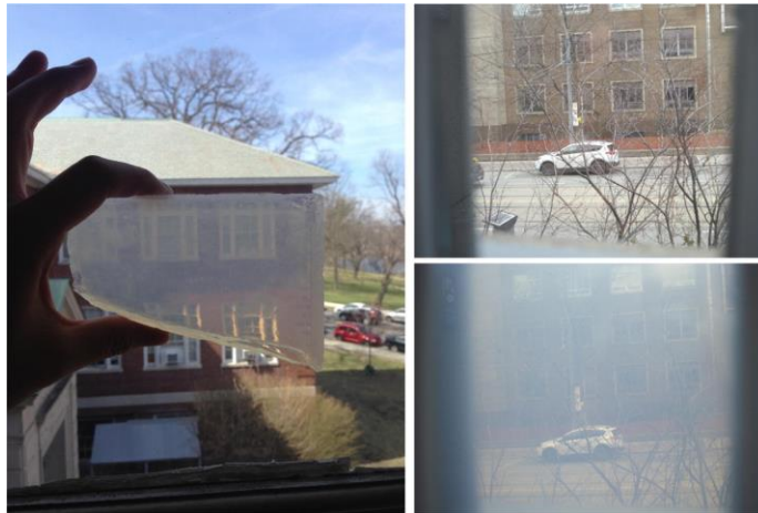
Figure 3: Sample of the monolithic aerogel panel used in the glazing units (Berardi 2015)
