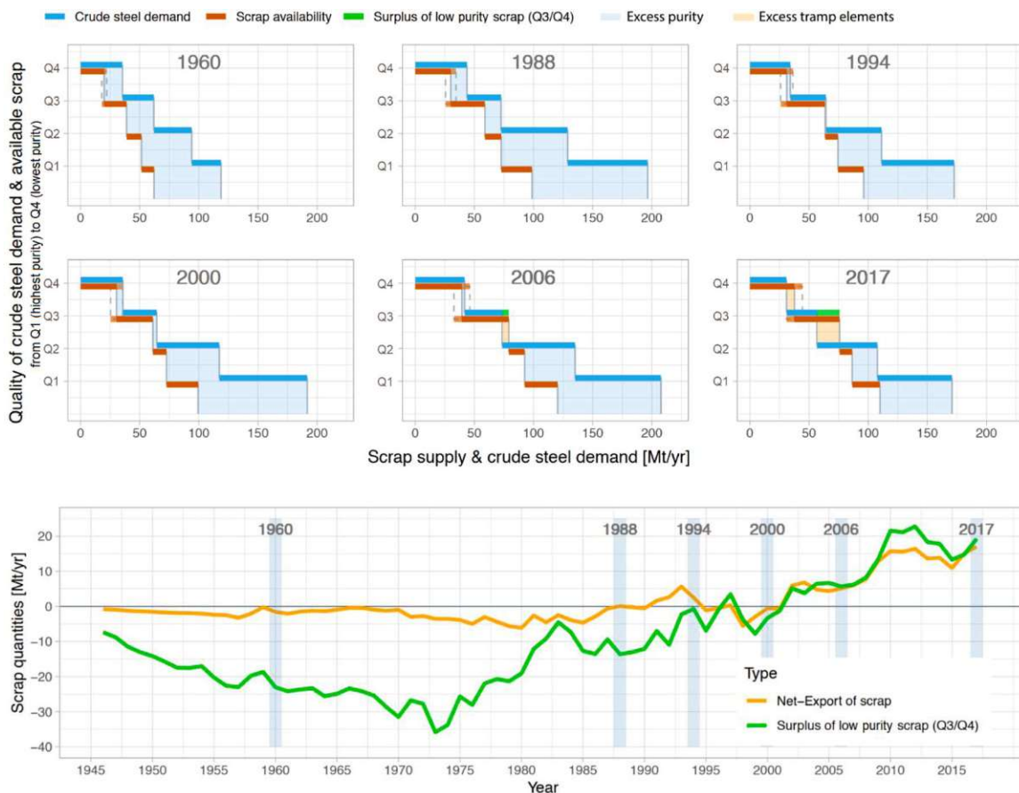
Fig. 5. Material pinch analysis for the quantities and qualities of crude steel demand and available scrap in the EU-28 for the years 1960, 1988, 1994, 2000, 2006 and 2017, orange-shaded areas show the excess tramp elements, blue-shaded areas the excess purities (upper part). Assessed scrap surplus of categories Q3 & Q4 and net-export of scrap from the EU-28 (data are given in Mt/yr). Starting from the time (mid-90s) when a surplus of scrap (positive values) occurred, a good match with the net-export of scrap can be observed (lower part). The overlap between Q3 & Q4 is based on the fact that the assignment of EoL scrap to these classes is uncertain (40% to 60% to Q3 and Q4, each).
