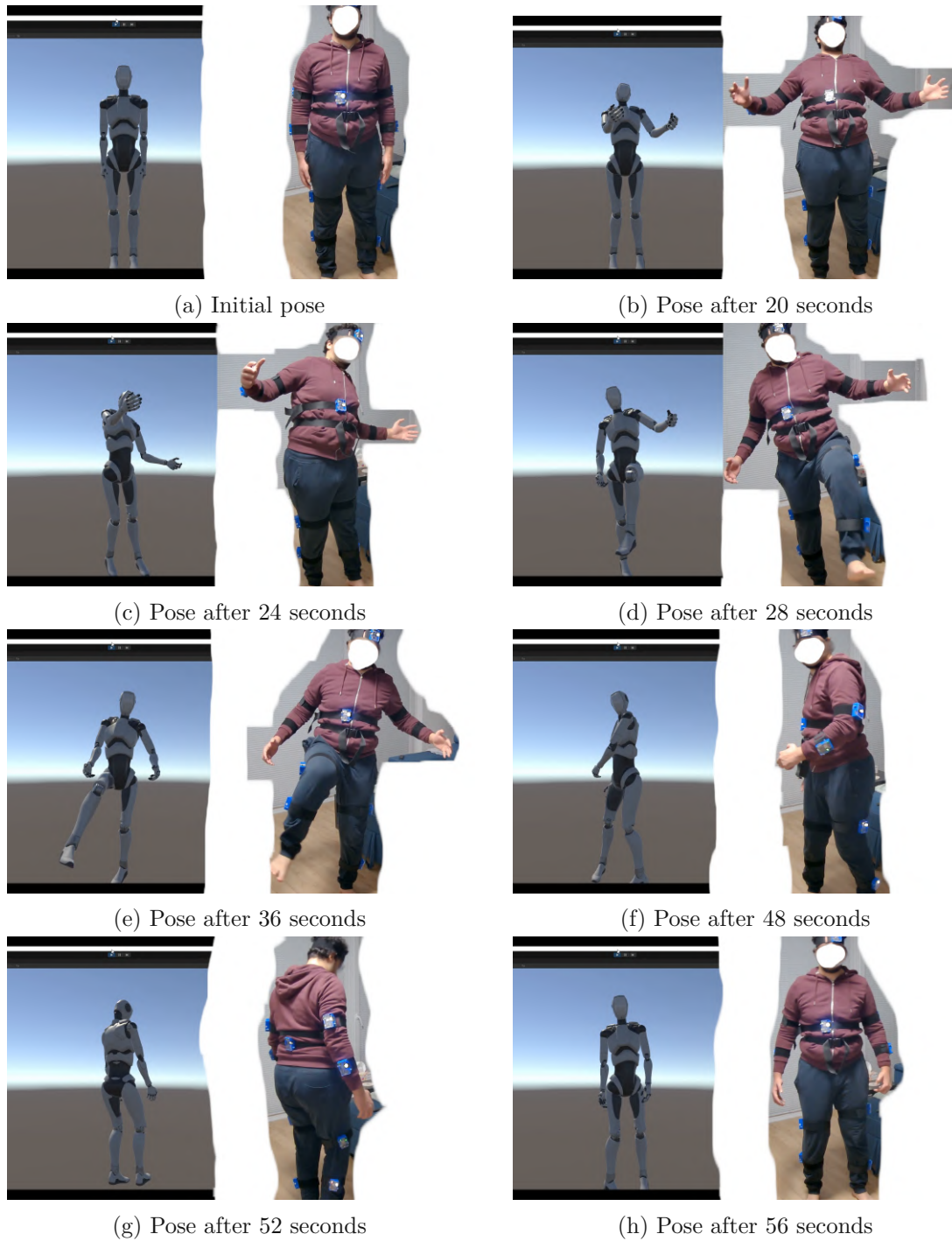
Figure 7.9: Shows a capture subject making slow body movements for 60 seconds as he is wearing my inertial motion capture suit. The real capture subject is shown on the right and the virtual humanoid 3D character in Unity is shown on the left side of the images.
