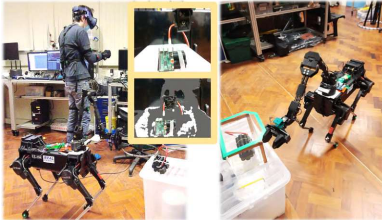
Figure 3.10: The user controlling the robot while wearing the inertial motion capture suit and a VR headset [ZPW + 22].
