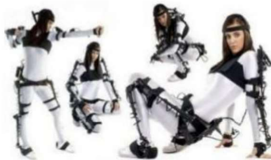
Figure 2.4: A mechanical motion capture suit (exo-skeleton). [Rah18].
