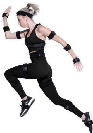
Figure 3.7: All 18 sensors attached to a capture subject using body straps [pns23c].
