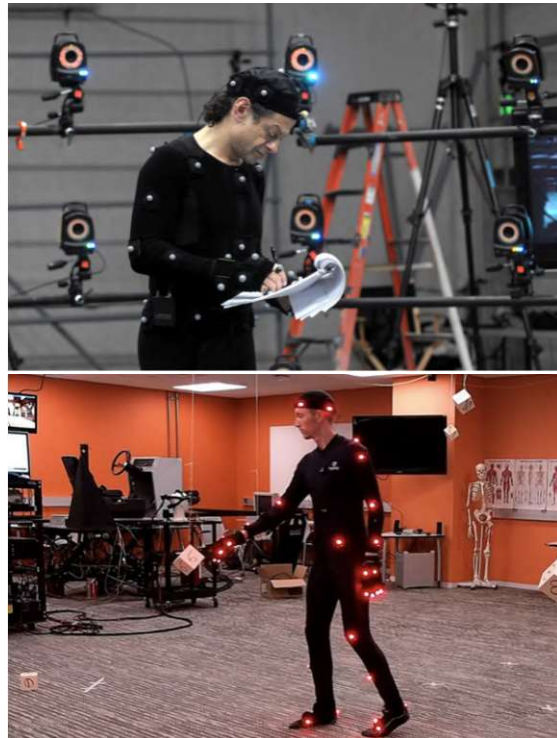
Figure 2.1: An optical motion capture system: Upper image shows a performer wearing passive markers and the lower image shows a performer wearing active markers [Ver21].
