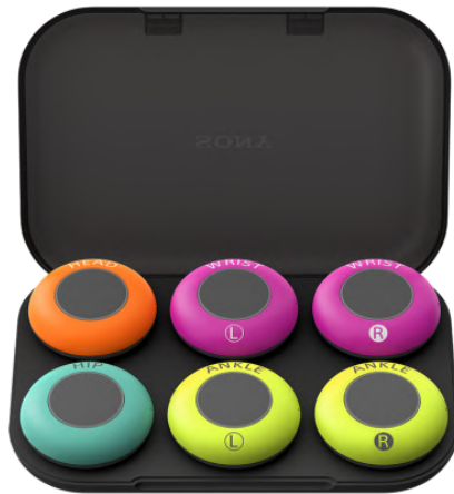
Figure 3.4: The six light-weight sensors where each one is assigned to a specific body segment [moc23b].
