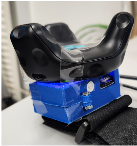
Figure 7.6: Shows the motion tracker attached to an HTC Vive tracker via tape.
